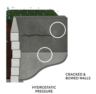
The pressure (or lack of support) often becomes too much for walls and causes them to crack or bow. Efforts to stabilize or reposition bowing walls should be taken as soon as possible. When cracks appear in these walls, the structural integrity is compromised.
